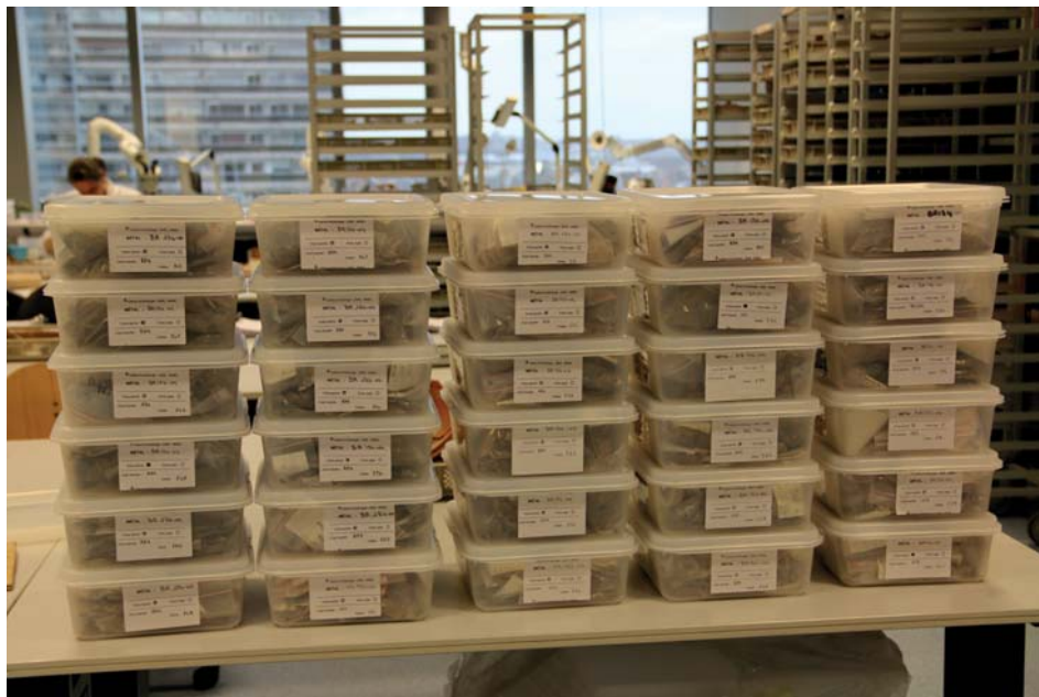
Figure 2. Preventive conservation applied to metal objects: a local climate is created in the boxes to prevent the metal objects to further deteriorate after been excavated (L. Cognard, 2017 © BRPS).
